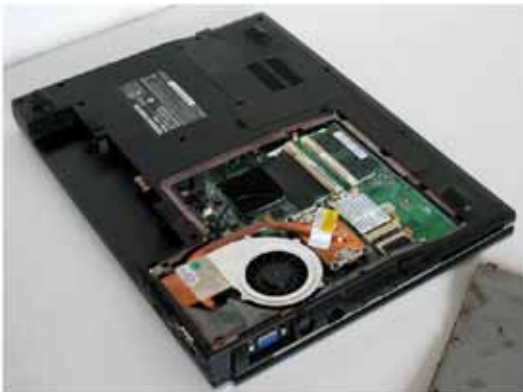
Figure 1 - Heat Pipe Cooling in Existing Notebook Computer [1]
