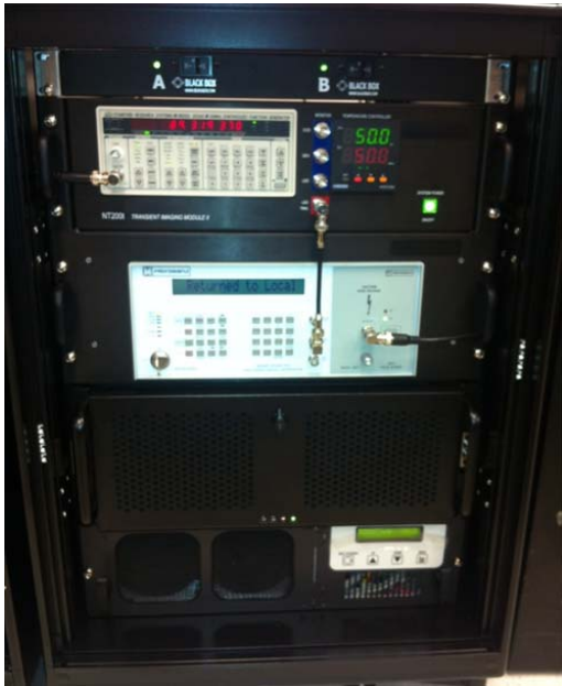
Figure 1: a) microscope and optical setup section, b) signal synchronization circuits for illumination, biasing, and imaging as well as data processing component of the equipment, respectively.
