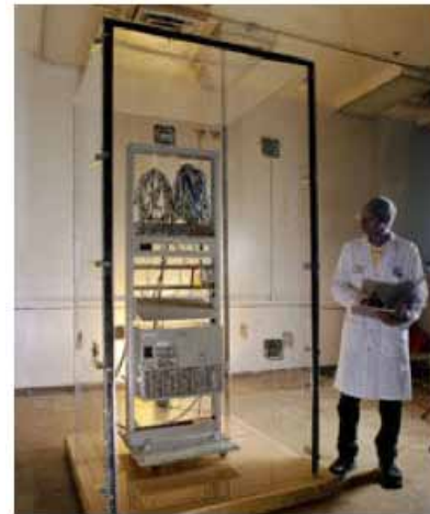
Figure 1 - Environmentally Controlled Chamber for NEBS Testing [1]
