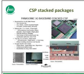
Or this example, where a two-die stack has been combined with high-density additive-technology printed circuit construction to create a package that is very little bigger than the chip inside, which is the source of the CSP acronym meaning "Chip-Scale Package".
