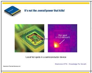
We have to remember though that it is not the overall power that kills, but local hot spots within the chip. This photograph shows a Pin Grid Array, with a bottom-up chip, and with the lid on the underside removed to make the die visible. In this case, there is an uneven heat distribution, and a corresponding hot spot on the chip. The stresses induced locally will be quite considerable, and may lead to early failure.
